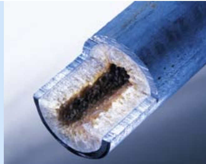
Don't put up with limescale deposits in your heating system – VDI 2035, Part 1, recommends the softening of filling and top-up water.
